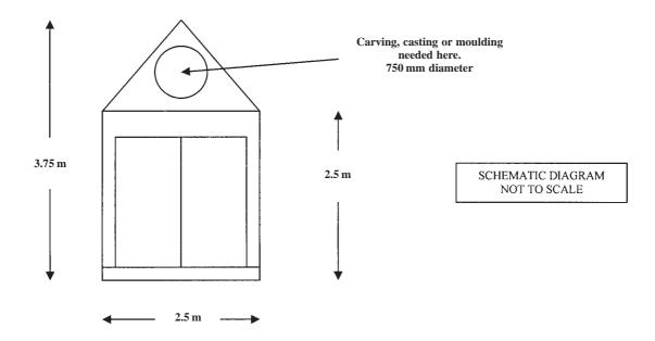
Create **two** sets of designs for carvings, castings or mouldings, that will be circular and be placed over the doors at the entrance to the proposed hostels in **both**:
