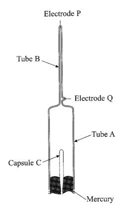
Radon gas,  $^{222}_{86}$ Rn, which decays by  $\alpha$ -emission to an isotope of polonium, Po, is placed at atmospheric pressure in a capsule C made from very thin glass. Any  $\alpha$ -particles passing through the glass from C become helium atoms in the evacuated tube A.
