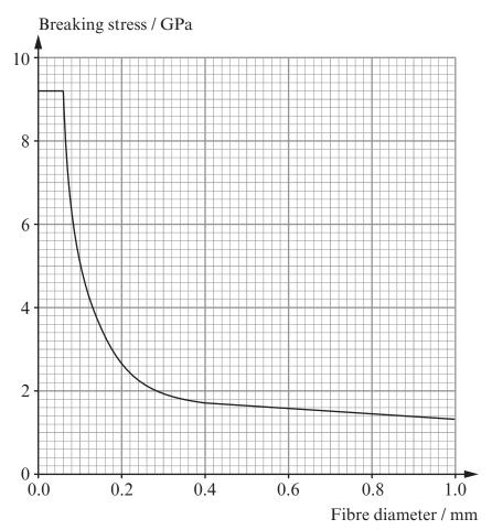
(a) Use the graph to estimate the greatest **mass** which can be hung from a glass fibre of diameter 0.20 mm. [2]
