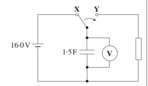
At time t = 5.0 s the p.d. across the capacitor has fallen to 8.0 V.
