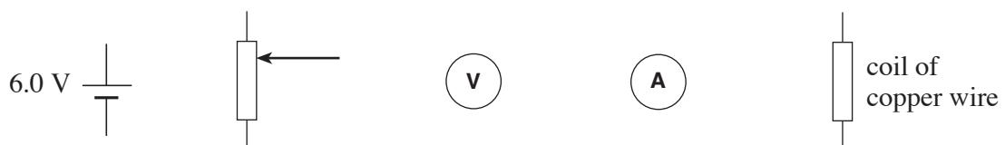
Draw a circuit diagram of the arrangement he sets up. The potential divider provides the full range of p.d.s between 0 and 6.0V.
