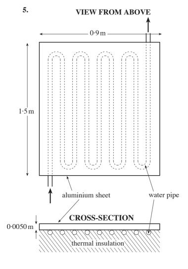
The diagrams show a simple form of 'solar collector' for heating water. A zigzag metal pipe is beneath, and in contact with, an aluminium sheet measuring  $0.90 \, \text{m} \times 1.5 \, \text{m} \times 0.0050 \, \text{m}$ .
