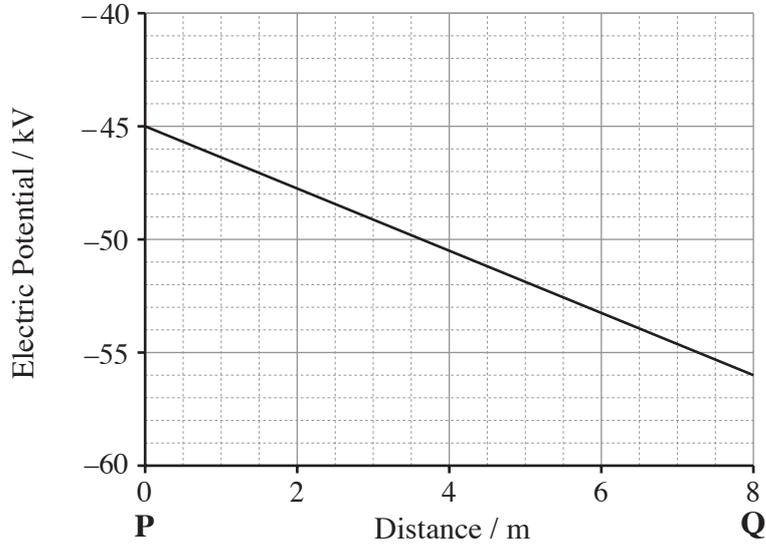
(i) Calculate the electric field strength between P and Q. [2]
