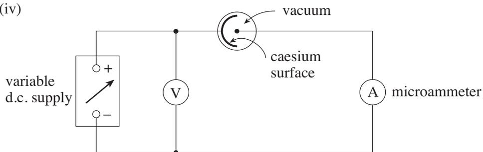
A vacuum photocell containing a caesium surface is wired into the circuit shown. The surface is illuminated with red light from the laser. State how the current changes as the size of the p.d. is gradually increased from zero. [2]
