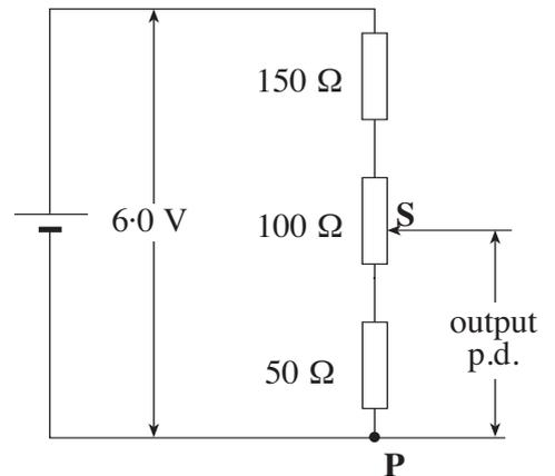
(d) **If the top and bottom resistors are replaced** the output p.d. can be made to vary between  $2.5\ \text{V}$  and  $4.5\ \text{V}$ , according to the position of **S**.
