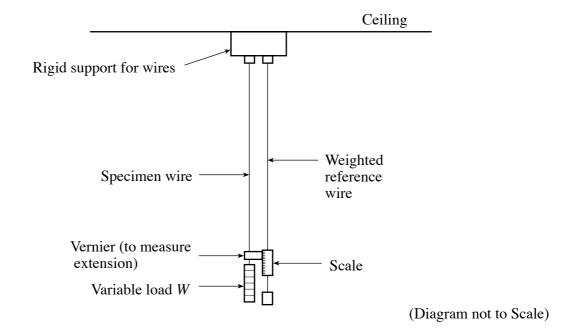
Successive extension readings are taken as the load on the specimen wire is increased but kept within the *elastic limit*. Readings are repeated during removal of the load, to provide mean values of extension. The length of the wire L is then found. A mean value for wire diameter d is obtained by making two measurements perpendicular to each other, with a micrometer, at a number of places along the wire.
