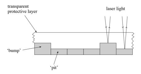
The CD is read using red laser light of wavelength 750 nm. The light is reflected from the metal layer and processed at a detector. When the light meets a 'bump' it is reflected and **interferes destructively** with light reflected from a neighbouring 'pit'. (For parts (i) and (ii) of this question, refer to the list of constants given on page 2.)
