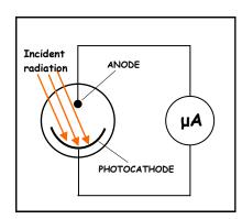
The **PHOTOELECTRIC** CURRENT, measured by the microammeter is proportional to the **number of electrons per second** which move from cathode to anode
