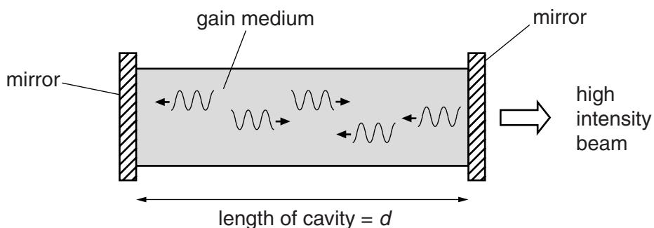
**Fig. 2:** the radiation reflects back and forth in the gain medium cavity, building up a standing wave
