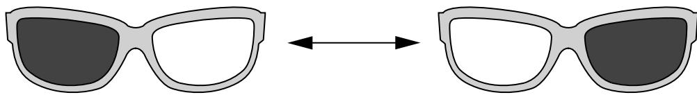
active 3-D glasses blank out left vision when the right eye frame is displayed on the TV
