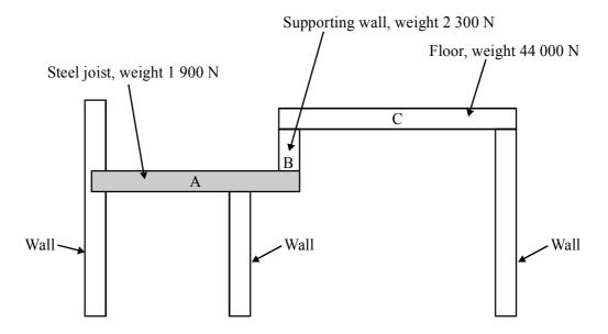
The steel joist A supports the supporting wall B and the left-hand side of floor C. Both the joist and floor C may be treated as uniform bars.
