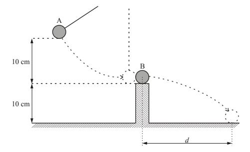
Sphere A is tied to the end of a long vertical thread and pulled to one side until it has risen a distance of 10 cm. It is then released and comes to rest when it strikes the sphere B which is resting on a smooth flat support.
