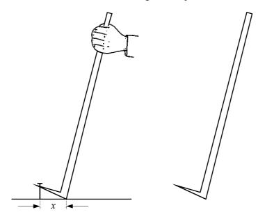
Use the diagram on the right to draw and to label a free-body force diagram for the crowbar. For each of the four forces which act on the crowbar, show the line of action, the direction and the source.
