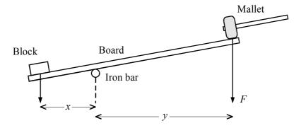
The block is thrown into the air when the right hand end of the board is struck by a mallet.
