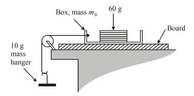
Add masses to the hanger until the matchbox *just* begins to slide. Estimate the total mass  $m_s$  in grams needed for this to occur. Hence find a second value for  $\mu$  given that
