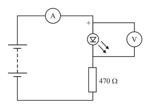
(ii) Connect the circuit to the power supply. Record the potential difference  $V_r$  across the red LED and the corresponding current  $I_r$ .
