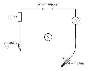
(ii) Connect the crocodile clip to the wire at the zero end of the rule. Connect the power supply and use the 4-mm plug labelled X to make a connection to the wire at the 20.0 cm mark. To make good electrical contact the 4-mm plug should be pressed **firmly** against the wire.
