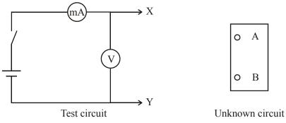
(ii) Connect X to A and Y to B to measure the current in and the voltage across the unknown circuit.
