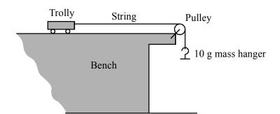
Add masses to the mass hanger until it is clear that the trolley accelerates across the table. Record the total mass m used to accelerate the trolley in the space below.
