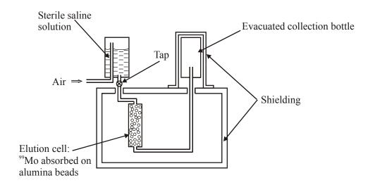
In which part of the generator is the <sup>99m</sup>/<sub>43</sub>Tc produced?
