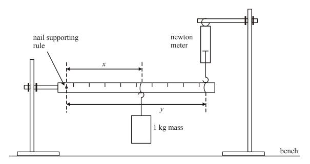
Adjust the height of the newton meter until the metre rule is horizontal. Explain how you ensured that the rule was horizontal. You may add to the above diagram if you wish.
