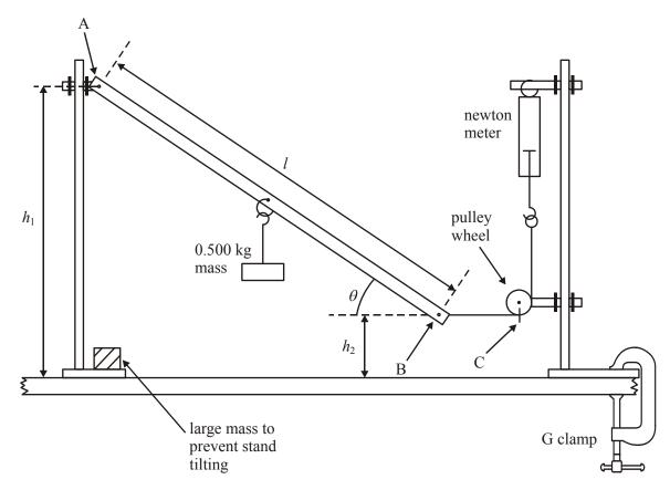
Do not move the stand that is clamped to the bench. Adjust the separation of the stands and the height of the nail at A until the section BC of the string is horizontal and the angle  $\theta$  is between 20° and 40°. You have been provided with a 30° set square so that you can easily estimate an angle in this range. Explain how you checked that BC was horizontal. You may add to the above diagram if you wish.
