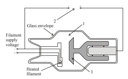
(iii) Name and explain the function of the numbered parts of the X-ray tube.
