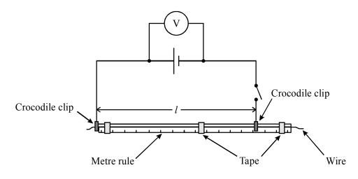
(b) You may assume that the voltmeter is an ideal voltmeter which takes no current. Use your circuit to determine the e.m.f.  $\mathcal{E}$  of the cell and the potential difference V across the length l = 0.800 m.
