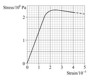
Use the graph to determine: the ultimate tensile stress for copper the Young modulus of copper **(3)** A copper wire of cross-sectional area  $1.7 \times 10^{-6}$  m<sup>2</sup> and length 3.0 m is stretched by a force of 250 N Will the behaviour of the wire at this point be elastic or plastic? Justify your answer. **(2)** Show this point on the stress-strain graph above. Label it P. **(1)** Calculate the extension of the wire.
