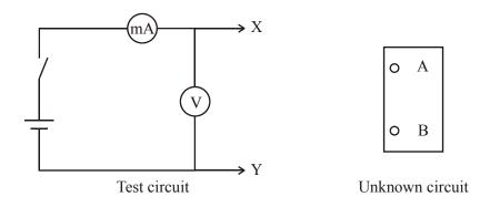
(ii) Connect X to A and Y to B to measure the current in and the voltage across the
