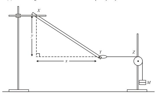
Adjust the height of the pulley and/or the position of the stands so that the string YZ is horizontal. Measure the distances x and y.
