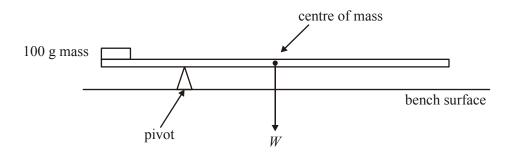
The centre of mass of the rule may be taken to lie at the 50.0 cm mark. Take such measurements as are necessary to find the weight W of the rule. **Show these measurements on the diagram.**
