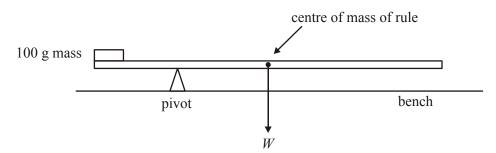
Take such measurements as are necessary to find the weight W of the rule. Show these measurements on the diagram.
