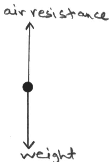
Ans = AS the velocity of the raindrop increases, air resistance also increases. So until so acceleration decreases. Then air resistance becomes equal to weight of the raindrop and resultant force becomes zero, so no acceleration and raindrop reaches a constant velocity which is terminal velocity.
