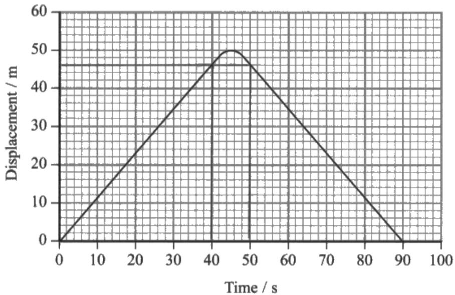
(a) Draw a corresponding velocity-time graph for the motion of the swimmer on the axes below. Show all working in the space below.
