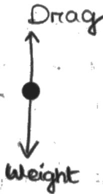
Terminal velocity is the velocity of the raindrop when all resultant force acting on it and all the result becomes zero.
