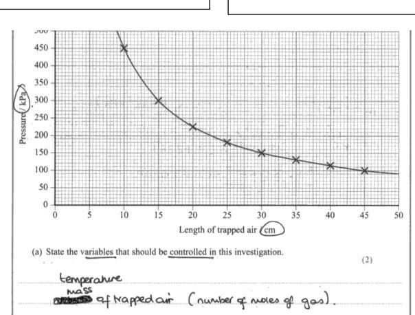
(b) Theory suggests that, for the <u>air trapped in the tube</u>, the pressure p is inversely proportional to the <u>volume V</u>
