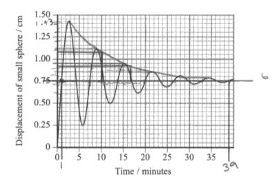
(i) Use the graph to determine the period of oscillation of the sphere.
