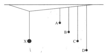
After a short time C is observed to have the largest amplitude of oscillation.
