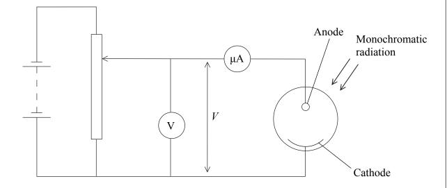
(a) When the potential difference V is set to zero, the microammeter indicates a small current. Explain how this current arises.
