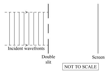
When wavefronts from the laser are incident on the double slit, interference fringes are seen on the screen.
