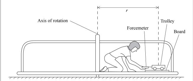
One student gets on to the roundabout and places a trolley on a board. The trolley wheels are parallel to a radius of the roundabout and the centre of the trolley is at a distance r from the axis of rotation. One end of the trolley is attached to a forcemeter which the student holds in her hand to keep r constant. She reads the forcemeter whilst a second student turns the roundabout at a steady speed. A third student times the rotations with a stopwatch.
