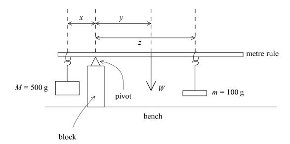
Place the pivot on the block of wood. Place the rule on the pivot at the 20.0 cm mark on the rule. Place one of the loops of thread at the 5.0 cm mark on the rule and suspend a mass M = 500 g from this point. Using the other loop of thread suspend a mass m = 100 g on the opposite side of the pivot. Move the position of the 100 g mass until the system is in equilibrium with the rule approximately horizontal. Determine the distances x, y and z shown on the diagram.
