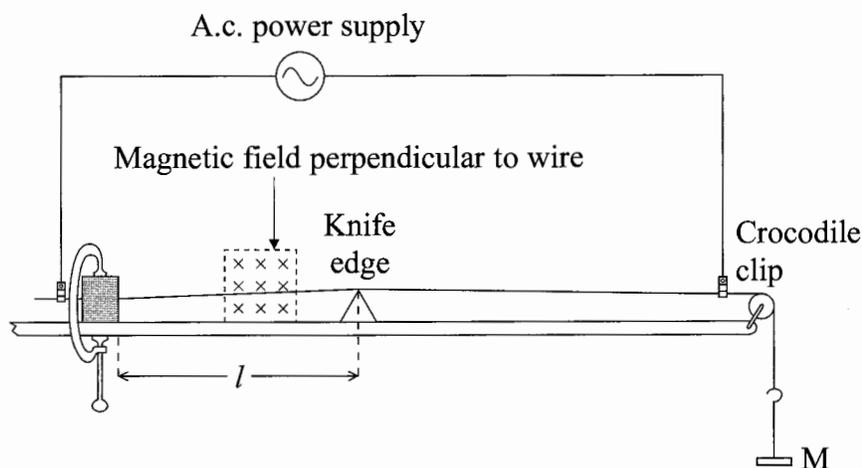
The fundamental mode of a stationary (standing) wave can be formed on a length  $l$  of the wire. Draw on the diagram the shape you would see. State the relationship between the wavelength  $\lambda$  of the wave and the length  $l$ .
