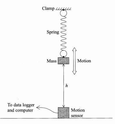
The data logger records how the height h of the mass above the sensor varies with the time t. The computer calculates the velocity v and acceleration a and displays graphs of h, v and a against t. Idealised graphs of h and a for two cycles are shown opposite.
