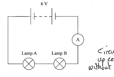
(ii) Connect the power supply and measure the current I in the circuit, I for I m H or better I = 0.055 A. | between 50 m A and 65 m A with wit (1)
