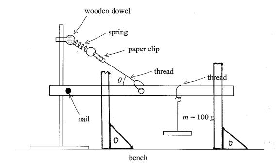
Adjust the height of the boss holding the wooden dowel until the metre rule is horizontal. Explain how you ensured that the metre rule was horizontal. You may add to the above diagram if you wish.
