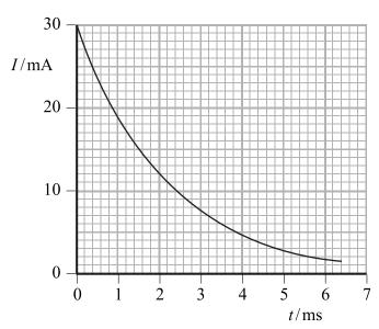
(i) By estimating the charge which flows, deduce the capacitance C of the capacitor.
