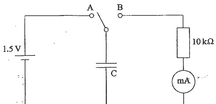
The capacitor  $C$  can be charged by connecting the switch to contact A and then discharged through the  $10 \text{ k}\Omega$  resistor by switching to B.
