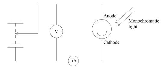
The photocell is connected so that there is a reverse potential difference across the cathode and the anode.
