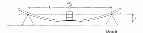
It is thought that for a given load, the depression x is related to the separation L of the supports by an equation of the form
