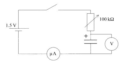
Set the variable resistor to its maximum value. Connect the spare lead across the capacitor. This short circuits the capacitor and discharges it. Once you have done this, disconnect one end of this lead.
