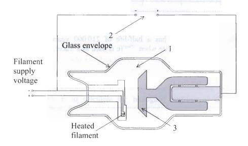
(iii) Name and explain the function of the numbered parts of the X-ray tube.
