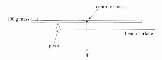
The centre of mass of the rule may be taken to lie at the  $50.0 \,\mathrm{cm}$  mark. Take such measurements as are necessary to find the weight W of the rule. Show these measurements on the diagram.
