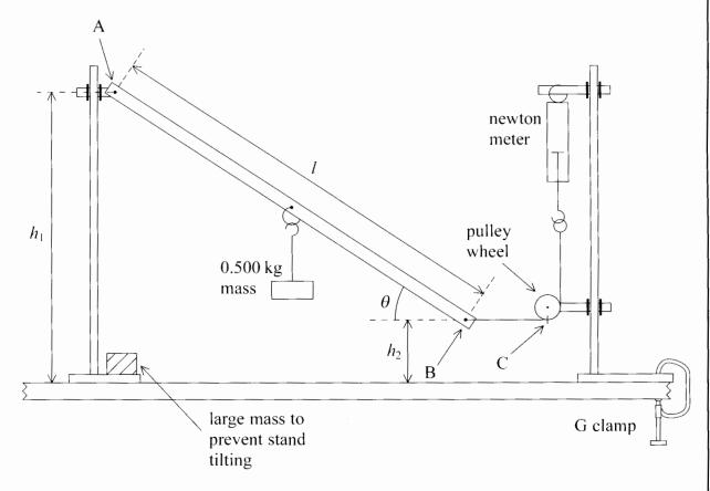
Do not move the stand that is clamped to the bench. Adjust the separation of the stands and the height of the nail at A until the section BC of the string is horizontal and the angle  $\theta$  is between 20° and 40°. You have been provided with a 30° set square so that you can easily estimate an angle in this range. Explain how you checked that BC was horizontal. You may add to the above diagram if you wish.
