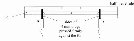
Measure the current I in the circuit and the potential difference V across the  $30.0\,\mathrm{cm}$  length of foil.
