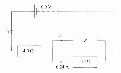
(a) Calculate the potential difference across the 15  $\Omega$  resistor.
