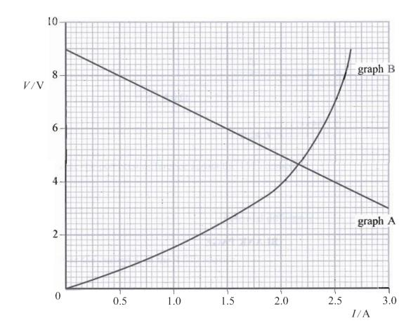
(a) (i) Use graph A to determine the internal resistance and the e.m.f. of the battery.
