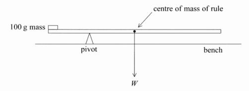
Take such measurements as are necessary to find the weight W of the rule. Show these measurements on the diagram.
