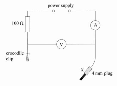
(ii) Connect the crocodile clip to the wire at the zero end of the rule. Connect the power supply and use the 4-mm plug labelled X to make a connection to the wire at the 20.0 cm mark. To make good electrical contact the 4-mm plug should be pressed **firmly** against the wire.
