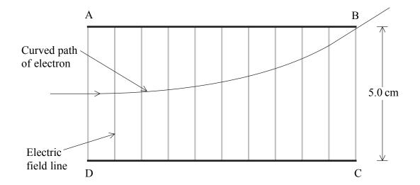
(a) Mark on the diagram the direction of the electric field lines.
