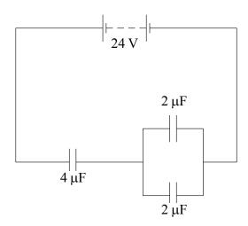
(i) Calculate the equivalent capacitance of the two capacitors connected in parallel.
