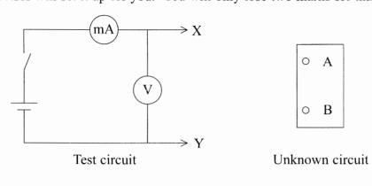
(ii) Connect X to A and Y to B to measure the current in and the voltage across the unknown circuit.
