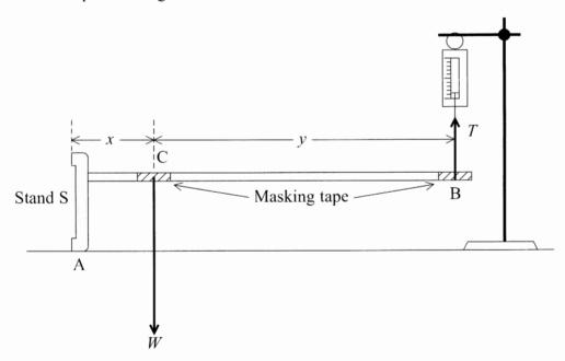
Support the rod with the newton-meter at a point B on the tape near the end. Mark this point.
