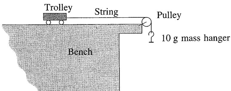
Add masses to the mass hanger until it is clear that the trolley accelerates across the table. Record the total mass  $m$  used to accelerate the trolley in the space below.
