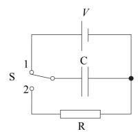
Switch S in the circuit is held in position 1, so that the capacitor C becomes fully charged to a pd V and stores energy E. The switch is then moved quickly to position 2, allowing C to discharge through the fixed resistor R. It takes 36 ms for the pd across C to fall to  $\frac{V}{2}$ . After the switch has been moved to position 2, how long does it take before the energy stored by C has fallen to  $\frac{E}{16}$ ?
