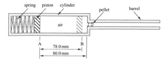
When the piston is at A, the air in the cylinder is at a pressure of 103 kPa and a temperature of 291 K. After the spring is released, the pellet remains in place until the piston reaches B.
