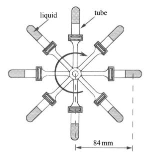
(a) When the centrifuge is operated with empty tubes, it reaches its working angular speed of  $1100\,\mathrm{rad\,s^{-1}}$  in a time of 4.2 s, starting from rest. The moment of inertia of this system is  $7.6\times10^{-4}\mathrm{kg\,m^2}$ . Calculate
