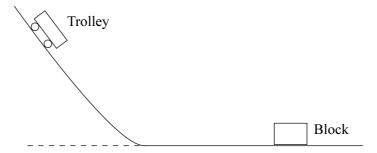
The trolley is placed on the raised section of the track. When released it moves down the track and then travels along the horizontal section before colliding with the block. The trolley and block join and move together after the collision. The distance they move is measured.
