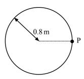
A model car moves in a circular path of radius 0.8 m at an angular speed of  $\frac{\pi}{2}$  rad s<sup>-1</sup>. What is its displacement from point P, 6 s after passing P?
