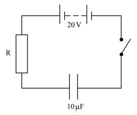
A capacitor of capacitance  $10\,\mu\text{F}$  is fully charged through a resistor R to a p.d. of  $20\,\text{V}$  using the circuit shown. Which one of the following statements is **incorrect**?
