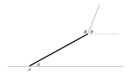
The coefficient of friction between the end A and the ground is  $\frac{3}{4}$ . Given that the end A of the beam is about to slip,
