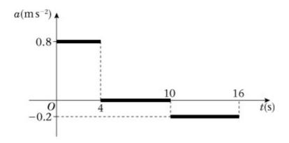
The diagram is an acceleration-time graph to show the motion of a particle. At time t = 0 s, the particle is at rest. Sketch a speed-time graph for the motion of the particle.
