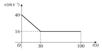
A train is travelling along a straight track. To obey a speed restriction, the brakes of the train are applied for 30 s reducing the speed of the train from 40 m s $^{-1}$  to 16 m s $^{-1}$ . The train then continues at a constant speed of 16 m s $^{-1}$  for a further 70s. The diagram shows a speed-time graph illustrating the motion of the train for the total period of 100 s. Find
