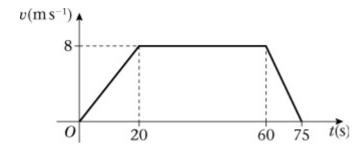
The diagram shows the speed-time graph of the motion of a cyclist riding along a straight road. She accelerates uniformly from rest to 8 m s $^{-1}$  in 20 s. She then travels at a constant speed of 8 m s $^{-1}$  for 40 s. She then decelerates uniformly to rest in 15 s. Find
