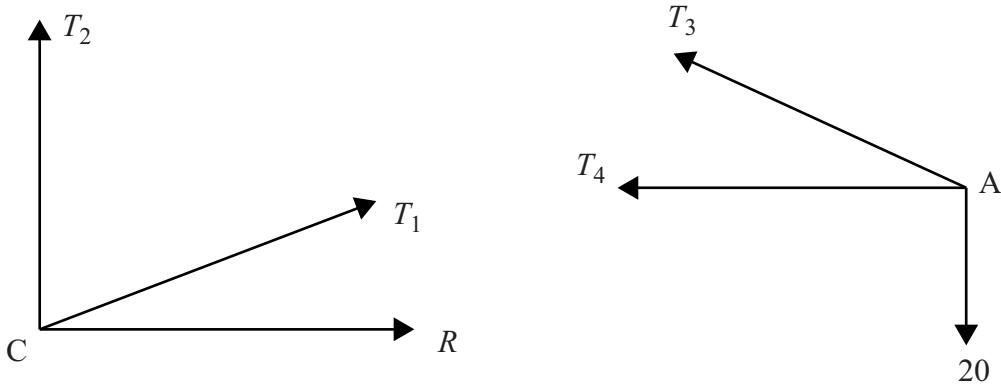
$T_1$ N,  $T_2$ N, are the forces in the rods meeting at C.
