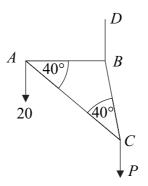
The rods AB and BC are of equal length, and the angles at A and C are each  $40^{\circ}$ . The framework is freely suspended from a fixed point D by a light rope BD.
