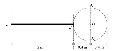
The pole AB has length 2 metres and mass 6 kg. The disc, centre O, has radius 0.4 metres and mass 2 kg. The points A, B and O lie on a straight line.
