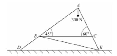
The framework stands, in a vertical plane, on rough horizontal ground. A load of 300 N is hung at A. The framework remains in equilibrium with BC horizontal. By considering the forces acting at A, find the forces in each of the rods AB and AC. (7 marks)
