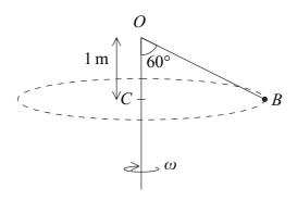
A ball B of mass 0.4 kg is attached to the other end of the cord. The ball rotates around the pole with constant angular speed  $\omega$  radians per second. It moves in a horizontal circle with centre C at a distance 1 metre vertically below O. The angle between OB and OC is  $60^{\circ}$ .
