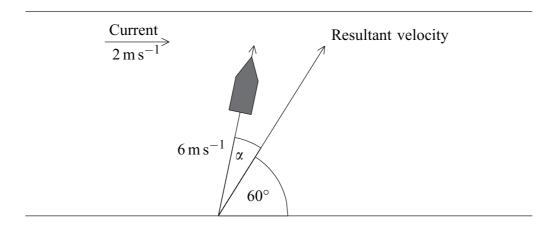
The angle between the direction in which the boat is travelling relative to the water and the resultant velocity is  $\alpha$ .
