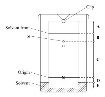
A pencil line was ruled on the chromatography paper to mark the origin. A concentrated spot of the solution was produced at X.
