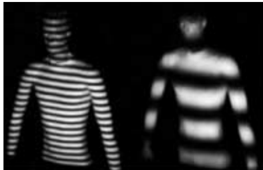
Figure 2: Triangulation between projector, camera and target subject
