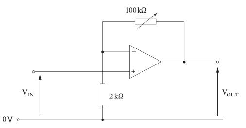
The op-amp is powered from a  $\pm$  15 V supply and saturation occurs at  $\pm$  14 V.
