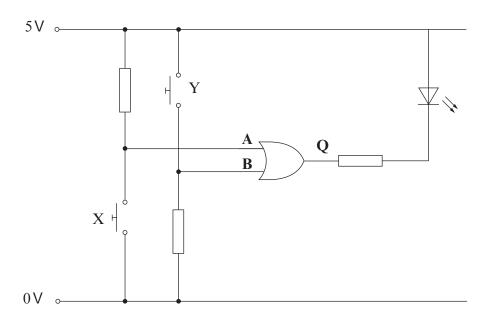
The table below shows the four possible settings of switches X and Y. Complete the table by adding:
