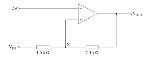
The circuit saturates at  $\pm 9 \text{ V}$ .
