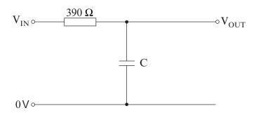
Show by calculation, which capacitor would be the most appropriate to use in this PCM transmitter. Choose from the following capacitors: 47 nF, 100 nF or 470 nF.
