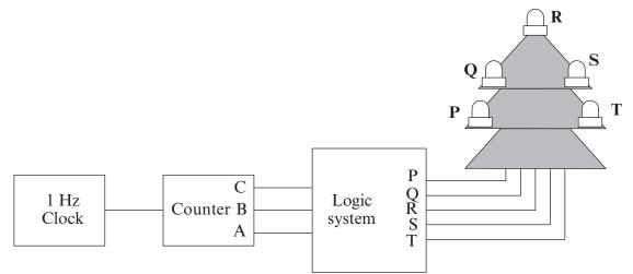
An LED is on when the corresponding output is high.
